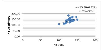
Fig. 1b: Scatter plot for Na<sup>+</sup> 9180 vs colorimetry
