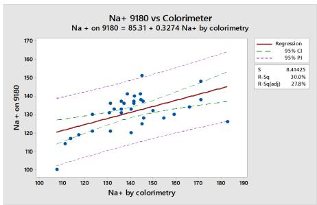
Fig 3: Simple linear regression for Na<sup>+</sup> values between 9180 and colorimeter
